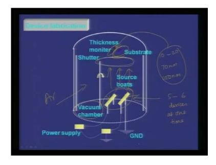
So, how to fabricate a organic device this is simple bell jar set up, which can be used for making this devices, and this is a vacuum chamber and in this vacuum chamber you have
