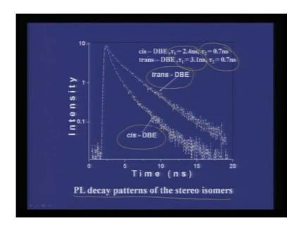
So, you can try to understand what really it takes and this is the photo luminescent decay patterns of the stereo isomers, as you would see for CIS DBE it is very, very different compared to trans DBE This can be fitted to a double exponential model where, both have nearly the same tau 2 values which is 0.7 nanoseconds, which comes somewhere here the linearity. But, you have the tau 1 values which are different, where CIS DBE has a much faster decay component compared to trans DBE.
