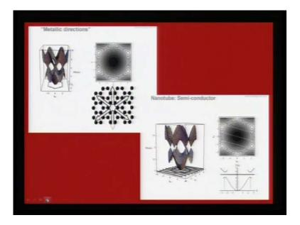
So, if you take the metallic directions and you try to map it, these are the six metallic directions, in which the electrical conductivity is confined. And in case of semiconductor carbon nanotubes or the graphene sheets, you see an opening of this band gap coming across the Fermi surface between the valence and the conduction band.
