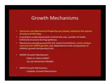
So, the growth mechanisms are very important to understand the electronic and mechanical properties, because both are dependent on the atomic structure of the tube. What we need to understand is that, what are the parameters that control the size, number of shells if it is multiwalled and the helicity and structure during the synthesis. What has been proved and established is that, there is no way you can grow a carbon nanotube without a metal catalyst.
