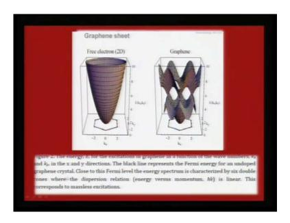
And if you look at the typical 2 D surface of a material, which is confined in two dimensional space, this is how it should look like. But, for graphene, you have a very different brillouin zone, that accounts for the conductivity of this graphene sheets.
