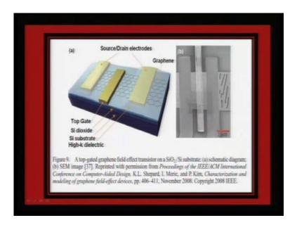
And graphene can also play as a very good metallic contact in transistors, field effect transistors. As you can see from this contour, you can easily make the graphite sheet, which is lying here. Graphenes can be made and then we can put a several electrodes for this transistor applications.
