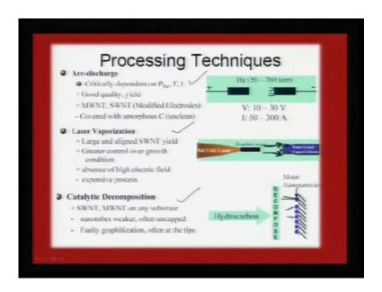
And we also looked at another view graph, where we said, there are three basic ways of preparing, one is CVD technique, another one is the arc discharge and also we have another technique using lasers. So, there are variety of ways, that we can realize this carbon nanotubes.
