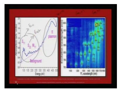
And when we come to the optical properties of single wall nanotubes, you would see a typical absorption peak for carbon nanotubes, where beyond 3 electron volt, this is due to Plasmon absorption. Whereas, there are peculiar reflections due to S 1 1, S 2 2, M 1 1, this S 1 1 or S 2 2 is actually to differentiate between metallic or semi metal carbon
