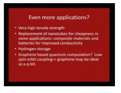
In terms of other applications, we can look for very high tensile strength and hydrogen storage also has been noted to be remarkably high for graphenes. Graphene based quantum computation is another thing, which is being probed now. I will just take you through few applications, before I finish.
