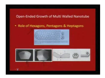
Open ended growth of multiwall nanotubes seems to occur mainly, because of the role of hexagons and pentagons, which played the important role in propagating this along one axis. As you see here, these are C 2 clusters, these are C 3 clusters and the way, they go and join to the nanotube, which is growing determines, whether it will be open ended or whether it will close or what will be their length scale of the growth process.
