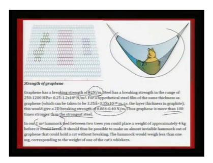
So, if you are actually going to spread 1 metre square of hammock like this, this is your hammock and if you are going to spread for 1 metre square, actually graphene sheet can take load up to 4 kg like putting a cat inside this hammock, so that much of strength can be derived out of graphenes.
