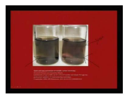
And the best part of carbon nanotube as I mentioned in the earlier slide, is the enrichment of this metallic carbon nanotubes. And we can also, not only enrich them, but we can go for preferential oxidation of this nanotubes to a larger extent. So, as you would see from this picture, that with more and more of selective oxidation, the color of this nanotube solution changes. So, these are those, which are oxidized which means, more and more of COOH groups are attached to the terminal carbon.
