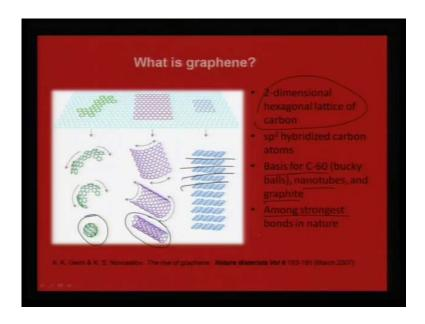
What is this graphene, the graphene as we pointed out, this is a two dimensional hexagonal lattice, from where we can either achieve this or this or we can actually get these layers of graphene. And this is the basis for C 60 for nanotubes and for graphite and among strongest bond in nature.
