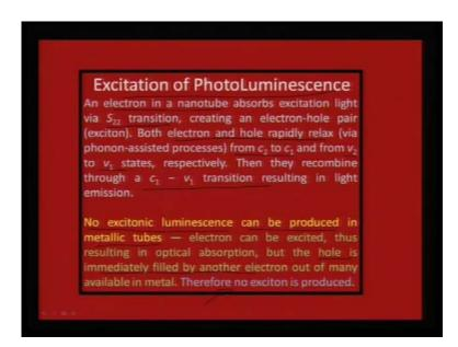
So, excitation of a photoluminescence, an electron in the nanotube absorbs via S 2 2 transition, as I mentioned earlier. And the electron and the hole rapidly relax from C 2 to C 1 and from V 2 to V 1, and therefore the C 1 V 1 transition is actually responsible for the light emission. And one thing that we need to understand here is, the photoluminescence is not due to excitonic emission, this is quite different from the other PL situation, where PL emission usually is an excitonic influence.
