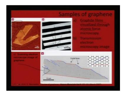
So, the graphene films are actually visualised by atomic force microscope and this is the way, it has been done. And as you could see here, the thickness of this graphene can be mapped using AFM and this is the TEM study, which clearly shows patches of graphene here. And here is the SEM micrograph of a graphene, which shows all the crystal phases of this film that is present, so it is possible to easily calibrate the thickness of graphite.
