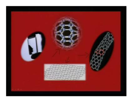
So, to conclude, we have actually seen three forms of carbon namely, buckyball then one dimensional carbon nanotube and also two dimensional graphene sheets.
