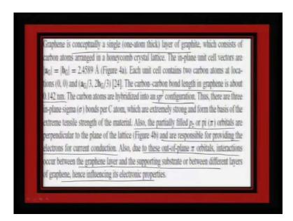
Graphene is actually a single layer of graphite, as we have seen and the carbon carbon bond in graphene is typically of this order and it is s p 2 hybridized. Actually if you see, we have partially filled p z or p pi orbitals, which are perpendicular to the plane of the lattice and these are responsible for providing electrons for conduction. So, it is more like a benzene ring, where your pi orbitals are perpendicular to the plane and your sigma orbitals stabilize the bonding.
