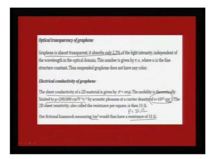
And therefore, it can be used for many mechanical applications, in terms of optical transparency it absorbs only 2.3 percent of light intensity. Therefore, a thinner graphene sheet say, 1 or 2 layers of graphene, almost will give you 90 percent transmittance, so it
