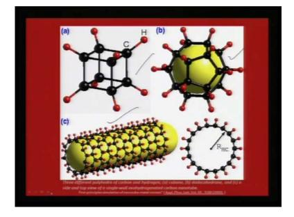
Now, this is a cartoon which is actually a simulation, but this shows the different polyhedras that the carbon can generate, and in this case you can see the three different polyhedra of carbon and hydrogen. One is a cubane type, another one is dodecahedron, and the other one is the carbon nanotube, this is exohydrogenated carbon nanotube, so this is out of a simulation that we have done developed just to show that there are three different polyhedras that the carbon can exhibit.
