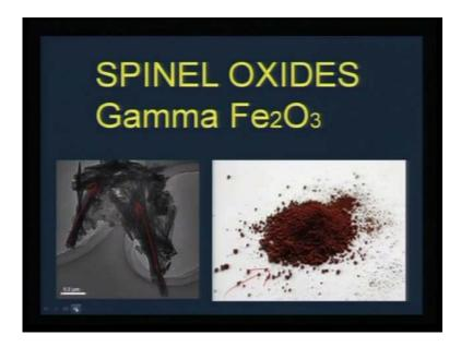
Another example is Spinel oxides, that is gamma Fe2O3, which is a very popular oxide, and usually it is reddish brown in colour. And gamma Fe2O3 is magnetic although
