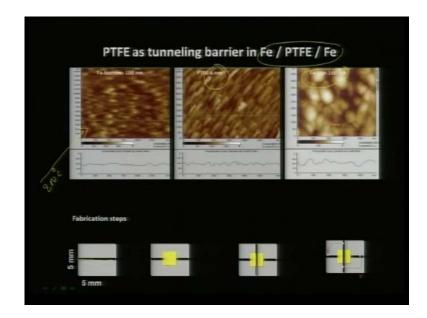
So, after ensuring that, it is possible for us to make a device structure of this configuration iron P T F E iron trilayer, how do you go about it, first you put a iron stripe like this and then we can put the organic layer. And then you can put one more metallic layer on the top and you can measure across the electrodes and then you can also see the A F M images of the iron layer, which is deposited as a bottom electrode.
