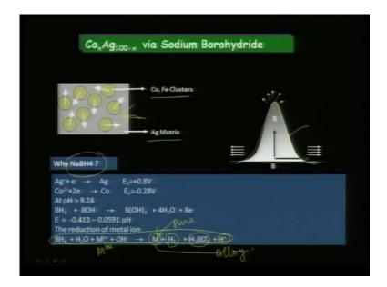
We can also look at the other granular system that is cobalt silver, again in this case you have the iron or cobalt silvers, which is dispersed in the silver matrix and we can achieve this sort of cobalt silver alloys by using sodium borohydride as the reducing agent. And this is the overall reaction, as to what happens sodium borohydride reacts with metal salts and it releases metal and boric acid and all this can be easily removed filtered, therefore essentially, you get a pure metal.
