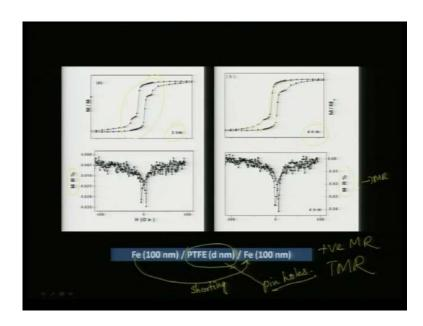
So, what does that mean, even though you have a 2 step magnetic hysteresis, there is shorting between the bottom and the top iron electrodes, it is short circuiting, as a result. We can say that this layer is not flat or it is not fully covered, there are pin holes in this layer, which is actually bringing about a short circuit between the top and the bottom electrode.
