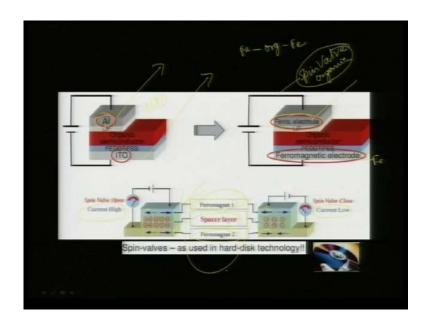
Now, how do how can, we translate the spin L E D into a spin magnetoresistive device, if you carefully look at this configuration, this is your oled device. And if you want to convert, it into a spin valve all you need to do is replace this anode a cathode and anode by ferromagnetic electrodes. So, if you replace I T O with a ferromagnetic electrode, if you replace aluminum with a ferromagnetic electrode, then you are essentially making a spin valve device, which involves a organic layer.
