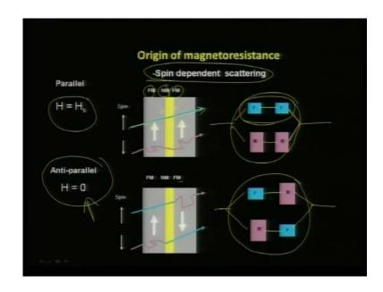
Now, just to bring back to focus, the 2 important mechanisms, that governs, we said if there is a ferromagnet here, which is aligned in this direction, ferromagnet here, which is aligned in this direction. And it is separated by a non magnet of this dimension, then you have 2 different resistance pathway, one is if the up spin electron is going from here to here, then you have a resistance pathway in this form and if you have a down spin, then you have a resistance pathway in this form.
