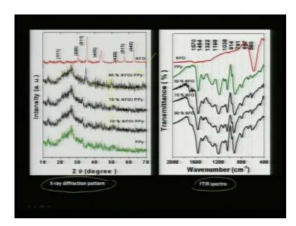
If you actually take a look at the infrared spectra and the x-ray diffraction spectra, you would find, it is very interesting that, the pure N F O, that is nickel ferrite gives a typical spinal pattern whereas, the P P Y, which is a polymer gives you amorphous pattern.
