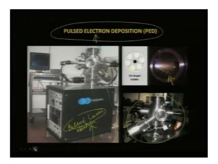
And what would happen in such situation, we can try to make this sort of organic layers using, pulsed electron deposition, which is a rugged facility and this is a typical pulsed electron deposition chamber, which has facility for a 6 target carousal. And you can use this pulsed electron beam to ablate the material from the target and typically during a ablation protocol, you would see the plasma, that is coming out.
