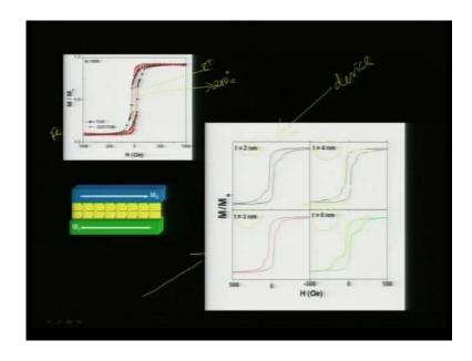
Now, how does the device respond, if you individually take the top and the bottom electrodes iron electrodes, you can see the coercivity is different, because when you deposit the iron at 200 degree C or so then the coercivity shrinks whereas, the top layer shows higher coercivity, which is deposited at room temperature. And this is the typical signature for the device, when device is there, then you would see, this 2 step hysteresis loop, which is showing the clear device operation.
