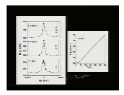
We can also try to do this with the iron silver alloy composites where, you see again a clear metallic behavior down to 4 Kelvin and one can see that, with increasing temperature the resistance increases and M R shows a very clear feature. Although the M R percentage is significantly low, but it is showing higher proportion at 5 K compared to 300 K.
