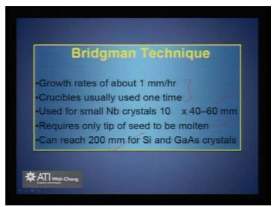
What you can achieve here is that crystals of dimension 10 to 40 millimeters can be realized, and it requires only tip of seed to be molten, which means a very small tip is needed, so that on that it can start growing. And you can also reach up to 200 millimeter for silicon and gallium arsenide crystals and this again is actually kept in a inert atmosphere, and some of the other issues from the economy point of view you cannot keep on using the same one.
