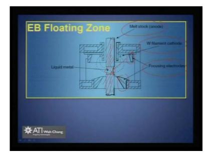
This is the typical assembly for this EB floating zone, where you can see here the tungsten filament cathode is there this is the melt stock which is nothing but your anode, so this has to be conducting in order to make this as a anode. So, this is your feed what we call and this is your seed with a interface and in between you can see the liquid melt which is actually melted using a filament, but in order to focus it only on this region otherwise the whole feed can melt.
