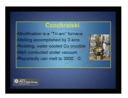
Czochralski method can also be modified and this is one such system, where you can see this is they use a tri arc furnace to quickly melt the feed, and melting is accomplished by three arcs then you can actually do a rotating water cooled copper crucible. And we can do this in vacuum, we can achieve up to 3000 degree C using this sort of tri arc furnace.
