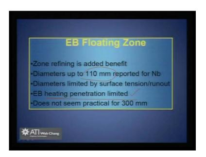
So, in EB floating zone you can get crystals of diameter up to 100 millimeter and then one problem that we face here is the penetration, it is not possible to actually run through the bulk especially when you have a feed, in EB what happens the surface melts, but then it does not really go into the bulk. Therefore, there are some practical problems which needs to be sorted out, when we go for this floating zone method.
