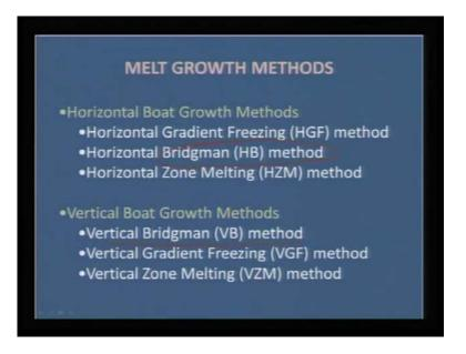
In melt growth method the most important one is a Bridgman technique, and this has a different way of realizing it, so you can actually go for a vertical Bridgman technique or you can go for a horizontal Bridgman technique. So, the assembly of your technique actually matters, but by and large the principle of Bridgman technique remains the same, we can also have the other one that is zone melting technique can either be in horizontal mode or it can be in a vertical mode.
