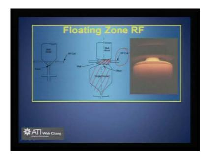
Here, is another picture of a floating zone apparatus where you are actually using a RF coil to melt this interface and here, again you can see the single crystal can be grown into a bigger dimension and that is one of the advantage of using a floating zone method.
