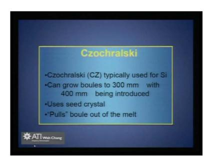
What is this Czochralski method this is a most industrially used method, because you can get very high qualities crystals, specially for silicon and basically this Czochralski method is even till now it is a sustained process, because the use of silicon is very important. Therefore, this is one of the established way to grow the crystal and you can see if you have a feed you can realize single crystal, successfully for three fourth of the batch that you are feeding.
