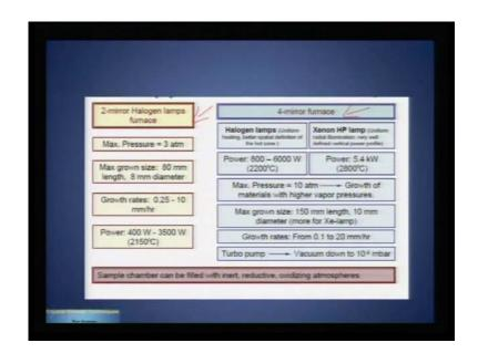
Now, to bring about a proper melting at the interface, there are different arrangements that are possible one is called two mirror a halogen lamp furnace, you can also have a four mirror halogen lamp furnace. And the whole idea in this floating zone technique is to make sure that it is really melting the zone in a very, very precise way without creating any temperature gradient over a large area, so lot of refinement has come into picture in this floating zone technique.
