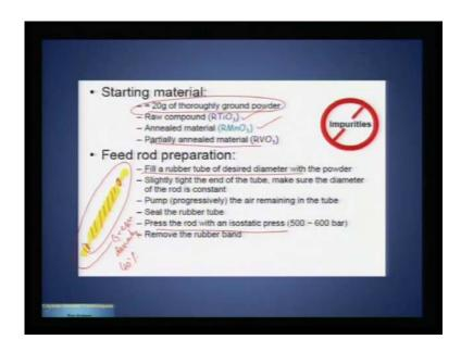
How do we go about this floating zone, simply we can start with an example roughly what you would need is about 20 gram of a powder, you can if it is a tight net you do not have to worry about it you can take the raw powder as it is. In case of manganites you need to actually anneal it little bit mainly, because manganites take carbondioxide or water it since it is reactive you need to activate the surface.
