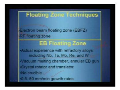
The next technique is a floating zone technique and here floating zone means you try to bring out a zone, which will divide between the feed and the crystal and the intermediate necking region is actually melted. So, how do you melt that you can use radio frequency to melt that region or you can use a electron beam to melt that region therefore, it is called EB floating zone a method.
