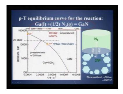
So, this is a typical profile of your pressure a temperature graph, which is required for achieving a gallium nitride formation using flux growth.
