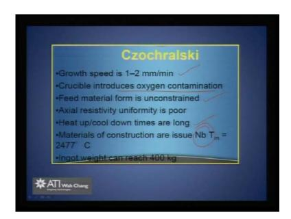
Therefore, the whole assembly has to withstand such high temperatures and then you can realize such single crystals, and the other parameters in Czochralski synthesis is the growth speed. Typically, you would not see the rotator moving because it is actually making an R P M very slow, so to your naked eye you would not even see anything moving, because you are actually going through 1 to 2 millimeters per minute.
