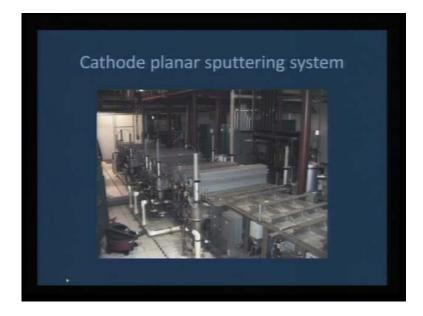
And as you would see here, this cathode planar sputtering is also a form of magnetron sputtering, how big this deposition unit can be you can easily scale it up to a industry level.
