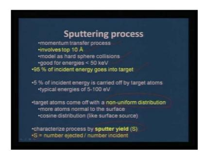
Now, in this sputtering process what is the parameters that we need to have in mind and what is this in effect, tries to convey to us. First of all it is a momentum transfer process, it is not a chemical reaction one ion with lot of kinetic energy coming and impinging on the surface of another target ion. And those atoms are actually removed, forcibly by the argon ions as a result top 10 angstrom of the atomic layer is actually replaced by argon atoms.
