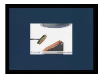
This is animation that will tell you the versatile nature of this sputtering process, as you would see here just by rotating or flipping the target, you can actually make multilayer's with these. And without breaking the vacuum, you can see both the green ones and the orange ones can be deposited with these. So, one of the main advantage of this sputtering process is you can do a variety of layer thickness, and you can change the material within
