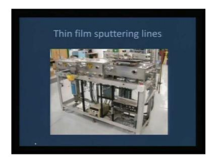
And this is one of the thin film sputtering lines, not just this we can even make a series of this into 6, 7 lines. So, scale up and transforming this into industrial process is very, very easy and in fact the silicon technology either you talk about solar cells or you talk about computer devices. The most adaptable technique as of now in the industry is the sputtering technique, because you can make large wafer depositions.
