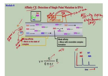
Now, like gel, we had worked on a different kind of capillary electrophoresis that is known as affinity capillary electrophoresis. Affinity capillary electrophoresis is ACE. Affinity capillary electrophoresis works on a principle that you have the capillary was electrode here electrode there. So, in the normal capillary you had buffer inside the capillary, before injecting the sample. In the gel, you had gel inside the capillary; they were interacting with your sample.
