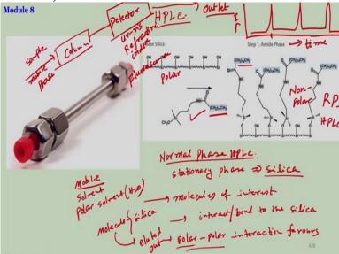
And we have talked about, so, this is your HPLC that such kind of column is being used, which is usually filled up with stationary phase in this case is silica. So, I have talked about reversed phase in the last lecture. So, there are many kinds of HPLC columns, it is based on different types of physical principles depending upon their physical properties, what of the material that is inside the column.
