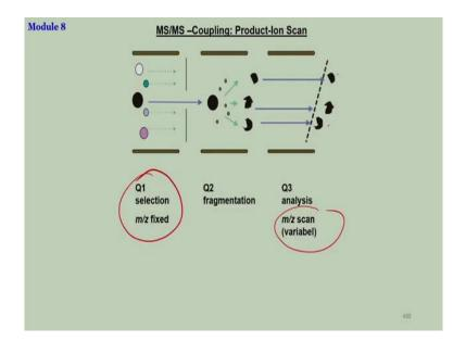
So, you have set of mass 1 2 3 4 5 for example. So, 4 quadruples are there. First quadrupol you fix a definite invoice it. So, only this is selected to go to that next quadrupol and here it will be fragmented. This is the fragmentation pattern of this particular mass. Remember all these mass is are actually a fragmented pattern from your earlier sample. So, this is the next phase MS MS phase we are talking about.
