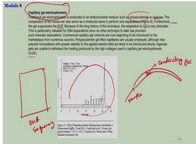
The capillary gel electrophoresis I have talked about that, in this case, you fill up the capillary with the gel. If this is your capillary, then capillary is filled up with the gel. Non-conductive gel of course conducting gel, so if you will now inject your sample across the capillary, it has to go through the gel. And obviously, if the sample has charged, gel has charged, so they will happen.
