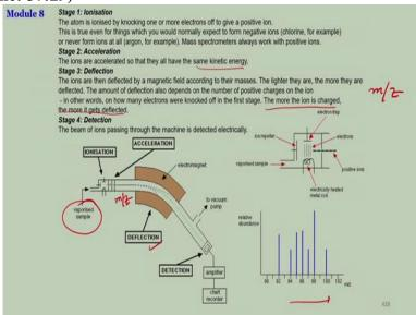
So, stage 1 is the ionization, the atom is ionized by knocking over one or more electrodes have to give a positive bias. This is true even for things which you would normally expect to form negative ions or never form ions at all. Mass Spectrometer always work with positive winds. Stage 2 acceleration the ions are accelerated. So, that they all have the same kinetic energy and then comes the deflection.
