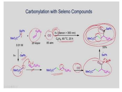
The first example involves the homolytic cleavage of the weak C-Se bond using light to produce the free-radical. The carbon radical bearing electron withdrawing ester group adds to terminal alkene to yield secondary carbon radical. CO trapping gives the acyl radical that reacts with phenylselanyl radical to produce the selenoate. (Refer Slide Time: 3:30)
