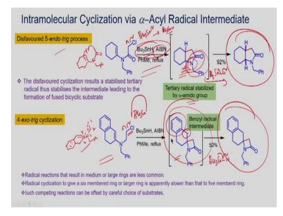
Here are two examples for the tributyltin radical mediated cleavage of C-Cl bond to form carbon radical. The first example involves *5-endo-trig* cyclization to give the bicyclic lactam. Similarly, the second example forms radical, which undergoes *4-exo-trig* cyclization to give the lactam.
