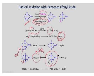
Here the diasetereoselective azidation of C-I bond of the bicyclic lactone is presented. Homolysis of 1,2-di-*tert*-butoxydiazene produces *tert*-butoxy radical. Which reacts with hexabutylditin to give tributyltin radical, which cleaves the C-I bond to generate carbon radical. Reaction with sulfonyl azide yields the alkyl azide. The azidation takes place to give a mixture of *syn* and *anti* stereoisomers.
