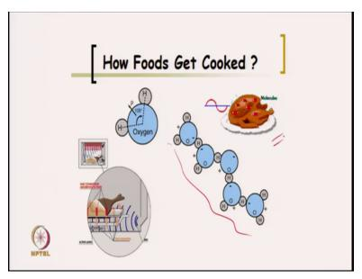
So, how food gets cooked is like this. Microwave Radiation is absorbed by water molecules. So, these are the water molecules and they basically absorb microwave radiation and what they do is when it is trying to come to ground state they do is by non-radiative emission. What does that mean is, it releases heat and then it comes back to ground state. This heat is used to cook food, is used to cook food.
