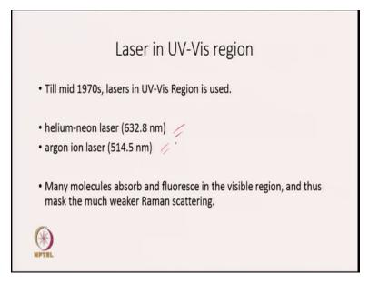
And initially lasers are used in UV-Vis region. The most commonly used was helium neon laser, which has wavelength of 632.8 nanometer and then argon ion laser which has wavelength of 514.5 nanometer. But problem with this kind of lasers are that many molecules absorb and fluoresce in visible region and the fluorescence will mask the much weaker Raman Scattering.
