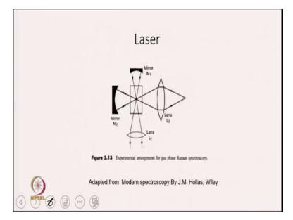
So, this is your typical experimental setup for Raman Spectroscopy, different lenses are used to focus, focus incident ray back to the sample.
