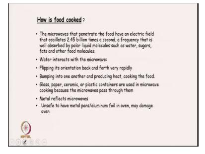
So, the microwave, that penetrate the food have an electrical field that oscillate, 2.45 billion times a second a frequency that is well absorbed by polar liquid molecules such as water, sugars, fats and other molecules.
