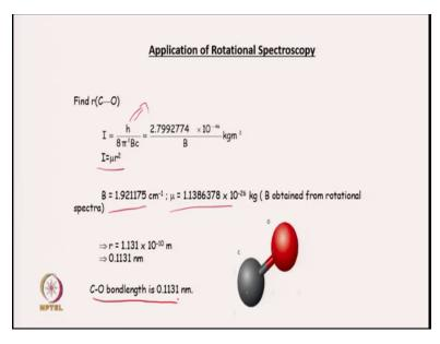
So, for example, if we take CO molecule, we can calculate CO bond length, if we can obtain Rotational Spectra of this molecule. From the Rotational Spectra what was observed that B is equal to 1.921175 centimeter inverse and by putting this into equation I is equal to h by 8 pi Square Bc, we can obtain your value of I and from I we can calculate your R since nu is equal to your 1.1386378 into 10 to power minus 26 kg.
