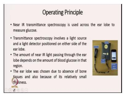
So, in this IR transmission your instrument is basically used across the ear lobe to measure glucose. So, you do not need a blood sample. And basically what is done is that a light source and a light detector is placed on either side of your lobe and then amount near IR light passing through the ear lobe depend on the amount of blood glucose in that region.
