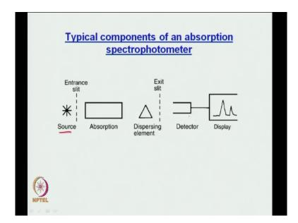
If you are doing an absorption, this is the typical component of an absorption spectrophotometer ok. The typical component of the absorption spectrophotometer has two things or few things, the first one is a source; source means you have to shine light, because it you remember the rho nu that energy density, you have to have that energy density, so that energy density comes from the source of the first one right.
