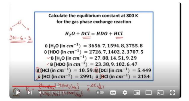
Rotational constant for water 27.88, 14.51, 9.29 non-linear rotor. Both H<sub>2</sub>O and HDO are non-linear rotor; therefore, you will require the values for A, B, C, 3 rotational constants.
