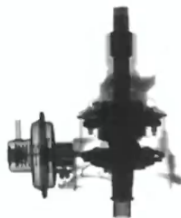
Radiography image of plug-valve
