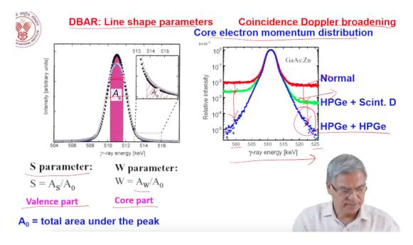
So in Doppler broadening, what is important is the line shape parameter. So this is a typical 511 keV gamma ray and you can see the 511 keV gamma ray FWHM will be here. So if the FWHM of a normal gamma ray is 1 keV, you will see it at 2 keV. You can see from 510 to 512. And so there are certain parameterization called S-parameter.
