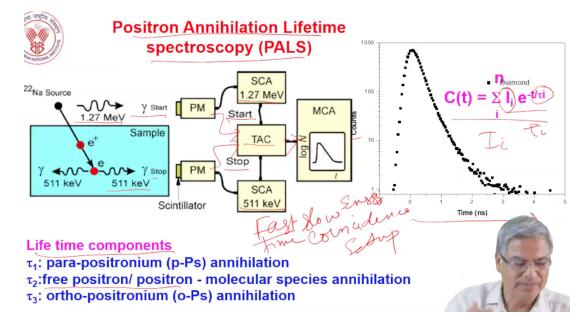
Another technique I was mentioning is the positron annihilation lifetime spectroscopy. And you measure the lifetime of a positronium or positron by a setup called fast slow coincidence setup, where this 1275 keV gamma ray from Na-22 source is triggering the start and the 511 keV are triggering the stop. So you have a circuit by means of which you determine the time difference between two gamma rays, 1275 and 511 keV. So what
