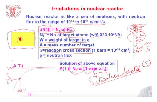
In fact, when you irradiate a target in an accelerator or in a reactor, how the active atoms are formed or you can even determine the activity. So if you determine the activity, you can determine the cross-sections. So first let us discuss how to determine how much will be the activity of a reaction product formed when you bombard a target with the neutrons or charged particles.
