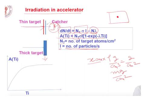
Now let us see the irradiation of targets in the accelerator. In the reactor, we have a pond like a pool, like a swimming pool, we have a lot of neutrons moving around and the sample is having very small dimensions. So all the target atoms are exposed.
