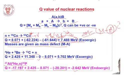
Now let us just go into the Q values of nuclear reaction, how to calculate the Q value of nuclear reactions. So simply again, I can write the reaction as A(a, b)B. So this is a projectile, the target, ejectile and the heavy residue. And the Q value can be given in terms of the (mass of the reactant - mass of the products)  $c^2$ . If you write in terms of the atomic mass units, then you would say  $\Delta Mc^2$ . And this Q value can be positive or negative.
