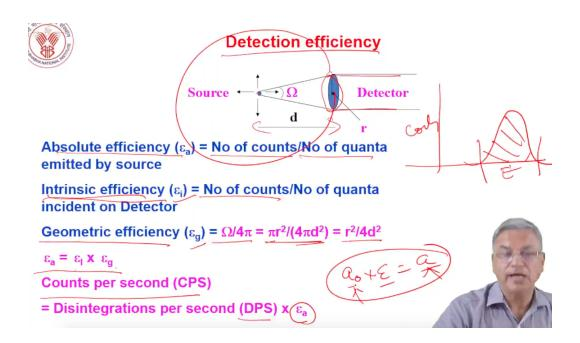
Another important property of detectors is the detection efficiency. How efficiently the detector can count your maximum radiations. So the radioactive sources, they will be emitting the radiation in all possible directions, in 4 pi. Though even if you put a collimator, then we are losing the radiation in other directions. So isotropic emission of radiation is the property of radioactive sources. They are emitting in all directions. But your detector has got a finite dimension.
