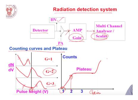
So this is a block diagram of a radiation detection system. You have a detector. It can be gas, solid, liquid. And you have to apply some potential. Somewhere ago the charged particles have to be collected at anodes and cathodes. So you apply the high voltage at the anode. And then once Q, the charge that is collected, you have to get a signal.
