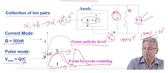
So how do we get the signal from detector? That is what we try to understand. So all of you know that Henry Becquerel discovered radioactivity simply using a photographic plate. So in essence, a photographic plate is also a detector. One of the oldest detectors is a photographic plate, but that will give you a qualitative picture.
