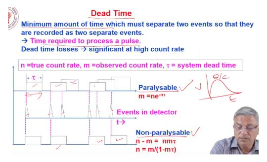
And the last thing property of detectors is the dead time. Dead time is when a detector is processing a particular event. During that time, it cannot process another pulse. So during that time, while it is processing one pulse, it is said it is dead to receive another pulse. So essentially the dead time is the minimum amount of time which must separate two events
