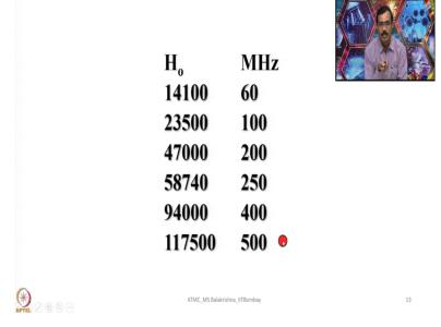
So, here I have given this radio frequency for different magnetic fields 14,100, it is 60 megahertz; this is with respect to hydrogen. And 23,500, it is a 100. So, this is how we have a 60 megahertz NMR, 100 megahertz NMR, 200 megahertz NMR, 250, 400, 500, 600 or even we have 1000 megahertz NMR now.
