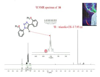
So, you can see here, this is a triazolic hydrogen coupled with two phosphorus atoms, as a result, it shows a triplet that can also be seen here. Also once if it is replaced and a metal comes here through CH activation, disappearance of this hydrogen can also be seen in <sup>1</sup>H NMR. So that concludes that yes, this hydrogen has been replaced and probably this ligand is acting as a tridentate ligand where we have a carbon to metal covalent bond.
