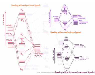
For comparison, I have put all the three types MO diagrams here. Clearly distinctly you can see the separation between these two and of course in this case, we also use the term HOMO and LUMO. This is highest occupied molecular orbital and this is lowest unoccupied molecular orbital, between which electronic transition takes place.
