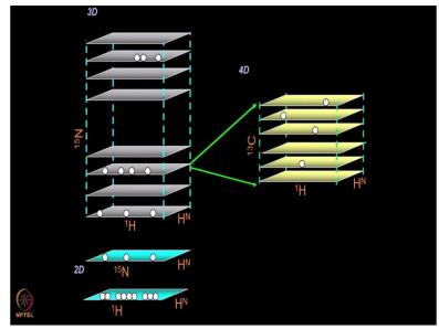
So, that is the schematic indicated here. So, you have the proton-proton correlation spectrum here, as we saw in the earlier spectra, then you also have the N15-proton correlation spectrum here, and then you would pull these peaks apart along the N15-dimension making use of the N15 chemical shifts here. There are three N15 residues, having the same amide proton chemical shift at this point.
