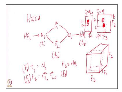
Let us try and draw this picture in a little bit more explicit manner. We are going to talk about the HNCA. So, we start from the amide proton of residue i and we transfer the magnetization to the nitrogen of residue i. So, here what we do is, we put a time label here t1, which means we are generating an independent time domain. So, the magnetization is evolving on the nitrogen and this is the t1 time domain, where the time is incremented systematically.
