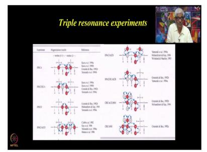
So, that is, therefore, you need 3 different kinds of nuclei and these are then called as triple resonance experiments, because they make use of proton, nitrogen and carbon-13. So, there are several sets of experiments which we have seen earlier when we were talking about the methods. So, we will now go back in a little bit of those details and try and explain how these things work some of those things will illustrate and the other ones can easily be followed thereafter.
