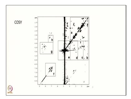
So, a whole COSY spectrum is shown like this here. So, this is the area of the amide protons and the aromatic protons, and you have the correlations in the COSY spectrum to the alpha protons here and then you also have from the aromatic protons to its beta protons and so on. Then of course when you go here then you will have the correlation from the alpha protons to the beta protons and then from the beta to the gamma, gamma to the delta and things like that.
