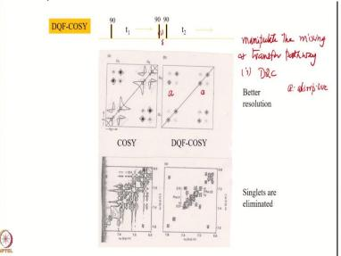
So, I have without going into the theory of this one we will see what is the final result? What is the result that comes out here? See here is this is the pulse sequence of the double quantum filtered COSY. So, you have the 90  $t_1$  90 of course here you can use the 90° pulse here this is up till here it is the same portion as the COSY. But we have introduced a small time delay here someone due to some small time delay that is a very small small very small time delay.
