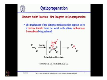
And this is the mechanism so it goes through the 3-membered transition state and followed by removal of zinc iodide. So, in the process zinc iodide comes out after delivering the CH2. And based on the evidence based on the products based on the mechanistic studies there was no free carbene involved in this reaction, always the metal was involved, the carbenoid was involved.
