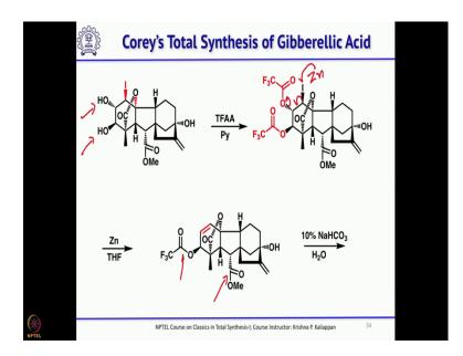
Then, what you need? You need to get a double bond for gibberellic acid ok. Protect these two hydroxyl which are trans to each other as trifluoroacetate, then treat with zinc. So, when you treat with zinc as you know zinc will give 1 electron and it can eliminate to give corresponding double bond. So, the lactone is formed and then, you have the O acetate, what you need is the ester should be hydrolysed. So, 10 percent sodium bicarbonate water.
