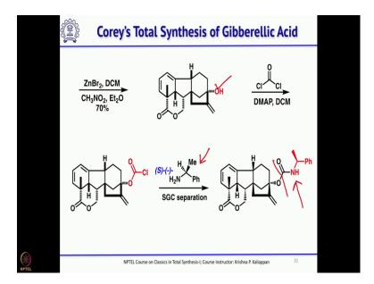
So, the next step is to remove the MOM group ok. So, you have a MOM group here; that MOM group was removed using zinc bromide. Then, if you use phosgene, it can form half ester ok. So, one equivalent of phosgene and then, this hydroxyl group, you form the half ester that on treatment with phenyl methyl amine ok. This is a good chiral resolving agent.
