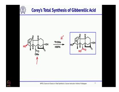
The trifluoroacetate could be hydrolysed to get the corresponding allylic alcohol. Then, the methyl ester, the hydrolysis of methyl ester is quite difficult. Because that is very unstable. The carboxylic as soon as the COO minus is formed, it is quite unstable. So, he has to use sodium thio propylate to hydrolyse the methyl ester to get the natural product.
