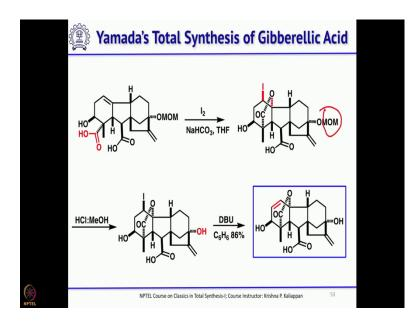
Then, you do metal ammonia that will cleave the CO bond; followed by acidification, you get this compound ok. Now, you do the iodolactonization once again, you get this and remove the MOM group with HCl and followed by treatment with DBU ok. So, DBU will eliminate the iodide to get the double bond and that is how Yamada completed the total synthesis of gibberellic acid.
