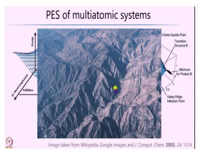
So, here what is shown is a potential energy surface for a triatomic system that is particularly water. And in this what you have is, one of the axis is that is typically the vertical axis is energy and the other two axes in this case the x and the y are in one case, it is the length bond length of the O-H and the other one is the bond angle, which is the again the two degrees vibrational degrees of freedom.
