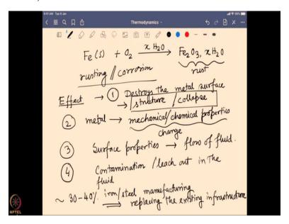
So, one most common example is if we take something made out of iron in solid form, and once it is exposed to aerial oxygen and water molecule present around in the form of humidity; it produces the iron oxide bound with water, and this is known as the rust. So, rusting is nothing but a corrosion process; so, why do we care about corrosion?
