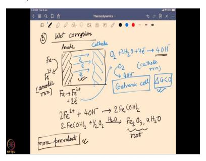
There is another process also happens at the same time, which is known as the wet corrosion. In the wet corrosion process, as it is quite obvious from its name; now the liquid or water has to play a big role. So, now say, I have an iron container and this iron container creates two different phases.
