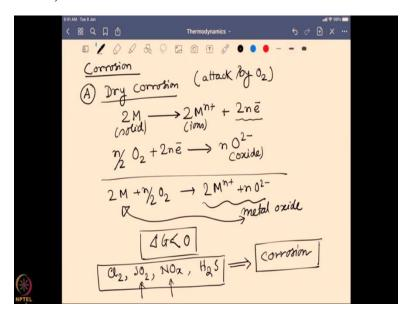
So, the corrosion occurs in two different ways. The first is known as the dry corrosion; so, I am taking the example of attack by oxygen. So, oxygen is present in nature in the air almost 21 percent is a strong oxidizing agent; and it will like to oxidize a metal present in its low oxidation state. So, what happens say metal is there present, it is getting oxidized; and it is giving electrons.
