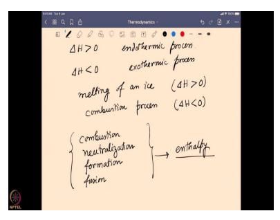
So, as we just said  $\Delta H$  greater than 0, it is an endothermic process and also  $\Delta H$  less than 0 it is an exothermic process. So, over here for an example, if we look into the melting of an ice, this has a  $\Delta H$  value greater than 0, so it is an endothermic process, so some energy has to be absorbed in that system.
