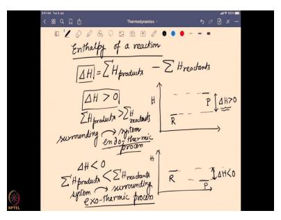
So, now when we talk about enthalpy, we talk about the enthalpy of a particular process, so let us say we are looking into enthalpy of a reaction, so how do I define an enthalpy of a reaction? So, enthalpy of a reaction is nothing but equal to enthalpy change during that reaction, and we can figure it out by adding all the enthalpy value of all the products we are forming, summing that up, minus all the enthalpy of the reactants.
