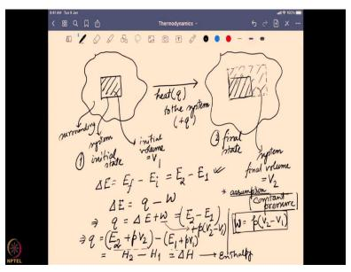
So, now say we have a particular surrounding and over there we have a system, where the system is expandable, say it is a gas. So, this system has an initial volume of  $V_1$ , then we are making some changes, in this full system where the initial system was this and now we are expanding the system, and now the system has increased its volume and we say it is the final volume after we completed that process is equal to  $V_2$ .
