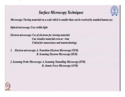
So, when we talk about surface analysis technique, one of the important techniques that comes to our mind is actually the surface microscopy. So, what is microscopy? Microscopy generally means that we can view a system or view a sample, in such a scale, which we cannot see by our naked eye. So, optical microscopy is quite common and it has well developed over the years by which, we can not only define the biological systems, but also material system.
