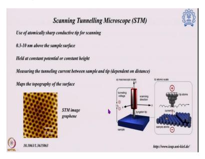
Then comes the probing microscopes. So far in the previous electronic microscope, we actually bombarded the system with electrons. Whereas over here, in the probing systems, we actually use a tip, a sharp tip, which actually can be handled in the atomic scale. And that is actually used for the scanning. So over there, I am showing you the picture that is how the instrument looks like.
