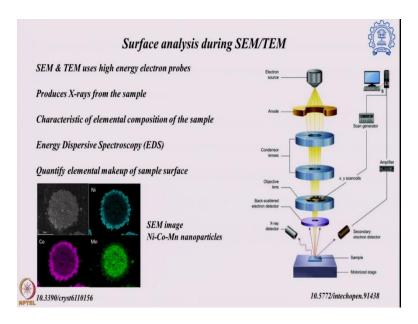
The good thing about SEM and TEM, as the high energy electrons are hitting these samples and as we just discussed a little bit earlier, it also takes out some electrons from the sample itself. And the electrons generally come from the core shell of the sample, so, they create a particular kind of X-ray, whose energy and signature will be very much different of which particular atom it is hitting there.
