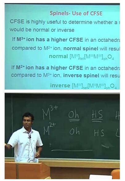
So, M3 plus ion has, when M3 plus ion has a higher crystal field stabilization energy compared to M2 plus ion then this is a normal spinel. If M2 plus ion has a higher CFSE then it is inverse
