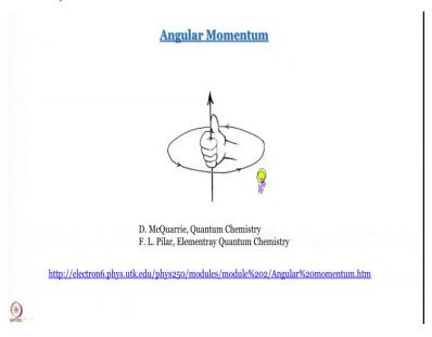
The quantity as such is not very new to us we are familiar with this kind of a diagram this is a cartoon that I have downloaded from this website. But in physics we have studied that whenever there is circular motion where the direction of motion is given by the direction of fingers of right. Angular momentum is a vector that arises perpendicular to the plane of rotation and is along the thumb of this right hand whose fingers are curled to tell us the direction of circular motion.
