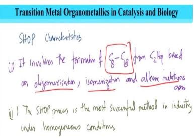
So shell higher ellucian process characteristics one it involves the formations of C8 to C18 from ethylene based on oligomerization, isomerization and alkene metathesis reaction. Now these we have discussed in detail in our previous slide where we had shown you diagrammatically where with example where each of these reactions play a role to produce this C18 to C8 to C18 fragments which are the application for detergent usage.
