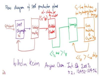
And that given by first ethylene feed so that would enter the oligomerization Jason chamber and then that would lead to the second chamber which would be used for catalyst recycling. So the Nickel catalyst used for shop would be recycled back for next phase then comes the distillation chamber which will give alpha olefin's for market and these would be C12 to C20 fraction C18 C12 to C18 fractions.
