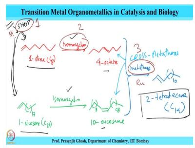
And this is based illustrated in the following slide for 1 octane octane and this is C18 fragment undergoing isomerization to give 4 octane. And similarly CH2 17 this is called 1 eicosene this is C20 fragments undergoing similar isomerization to give C8 this is called 10 eicosene fragment which after isomerization would be subjected to metathesis to give C10 C14 fragment which is called 2tetra disene and this is the D14 fragment.
