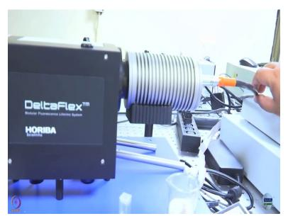
Let me show you the detection channels. The first piece of optics through which the emitted light goes through goes is a polarizer that is kept here. This is a polarizer put it in here we have a monochromator which we have discussed in the theory class and this is a fast detector that we have it is a new kind of hybrid detector and you can see the output of the detector goes through this thick cable.
