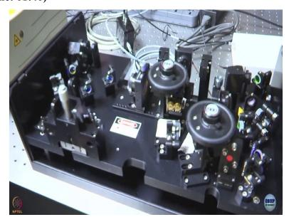
Now, the titanium sapphire laser gives us output as I said in the range of 690 nanometer to 1040 nanometer, which is basically red almost near IR kind of range. This wavelength is not really useful for excitation, if you are going to talk about fluorescence experiment. Secondly, the repetition rate at which the pulses come out of the laser is about 80 megahertz or 100 megahertz, you can think, which means the separation in time between two pulses is about 12.5 nanosecond.
