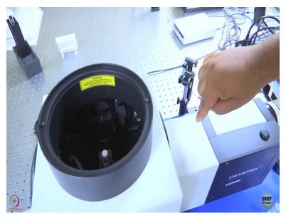
So, we have kept our sample in this cuvvette and that goes in here. So, excitation light comes this way, hits the sample emits in all directions, but we record in a perpendicular direction.
