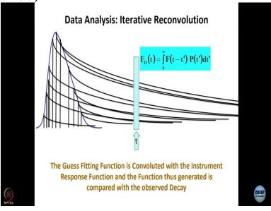
Let us think of a laser pulse of a finite width. So we can think that every point on this envelope is the tip of a delta pulse right and how many delta pulse would be there under this umbrella in principle in finite in theory and finite in practice, the number will actually be finite because as we discussed already we work with some picosecond per channel resolution. So, depending on how many picoseconds are covered under this curve.
