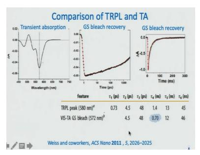
This is a comparison between time resolved photoluminescence and transient absorption fitted independently and that is the beginning of the story. Fitted independently they get a very good match. First of all where did 6 time constant comes from 3 came from one experiment 3 came from another experiment in PL itself. Now when they do transient absorption again picosecond and nanosecond they get actually the same time constant.
