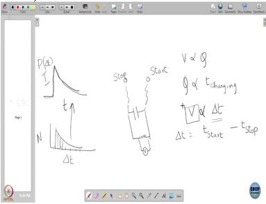
So, if I can try to draw it a little bit. So, what you have is this, let us say this is stop let us say this is start this signals go into starting of a capacitor the start and stop starting of the capacitor when it is stop after that, the capacitor is discharged across this resistance and you measure the voltage across the resistance. So, now see do you agree with me that the voltage that you see is going to be proportional to the charge that has accumulated on the capacitor.
