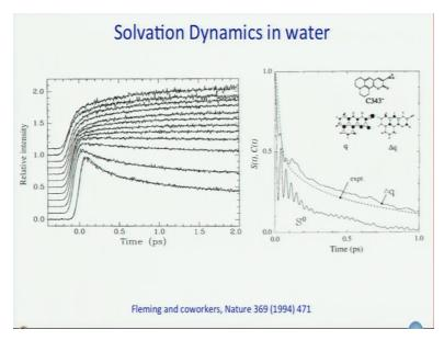
So this is this has become one of the most used fluorescence probes after this study ok. So there are coumarin 120 is 1 343 is 1. So using this Fleming and coworkers got this kind of time resolved decay. This is all femtosecond optical gating experiment ok. You can see fast decay in the blue end rise in the red end and you can note the full scale of the experiment 2 picosecond. Of course this is zoomed in picture they did not do the experiment for much longer time.
