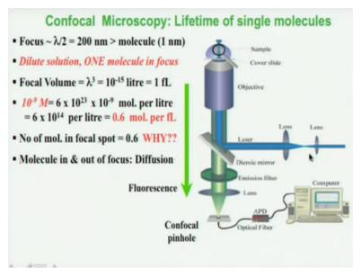
In which they used confocal FLIM set up so this is lifetime imaging microscopic set up. When I say confocal what it is essential means is that this is where you are sample is right. So the excitation light is focused on to a particular point in the sample focal point as you know cannot be less than Lambda by 2 in diameter that is the diffraction limit. And then there is Dichroic mirror that sends
