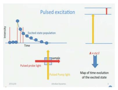
Okay now fluorescence is not the only technique that we have studied the commonly used technique which we have whose components we have studied in great detail is pump probe or transient absorption. Here what you do is you excite your sample by a laser pulse an intense laser pulse which causes an excitation to some higher excited state. And then what you do is you look at the excited state population that is going to decay with time.
