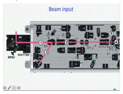
So here you can see this is the beam input pathway. It comes in like this is what the beams splitter looks like from the top this is a second mirror and then you go straight this is L1 this is L2. These lenses are actually mounted on cylinders and in principle you can move them back and forth you should not unless it everything is broken and you have to and you know how to fix it.
