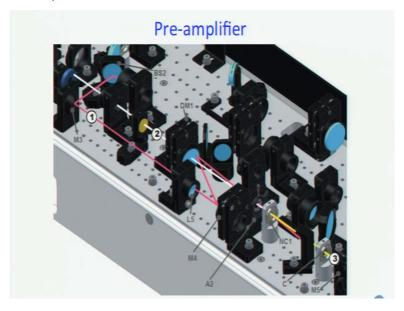
Moving on this is the isometric view of preamplifier once again if you have seen TOPAS you will be able to compare the optics and know which is which?
