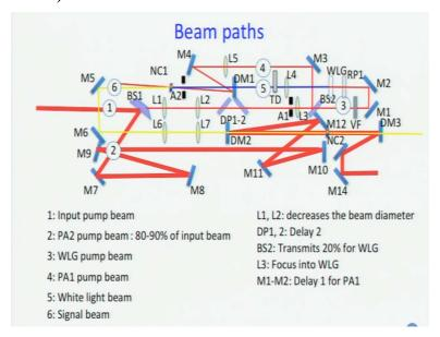
So this module to hope to complete our discussion of an actual optical parametric amplifier the one we use in our lab. We have this is where we are this is where we go to until the last module. To recap quickly we have this input beam hitting beams splitter 1 80 to 90% of which is reflected on to M7. Remaining part of it goes straight using L1 and L2 pairs of lenses which constitute a telescope.
