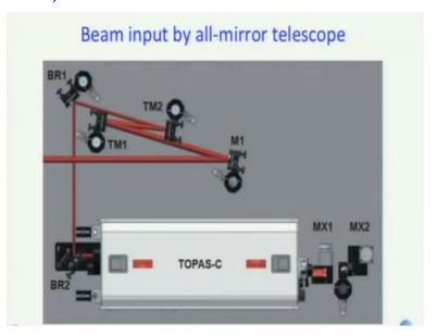
We are discussing a the optical parametric amplifier we have in a lab TOPAS C. What we have said so far is that we put in the beam the pump beam output of the part of the output of the regenerative amplifier we have using an all mirror telescope. And the reason why we need so many why do we need so many mirrors let me ask you? Yes one is path length you might have to give a particular delay because later on some other application right.
