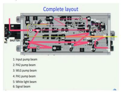
And this is what we have shown you we said that you have light coming in from the regen and using beam splitter and different optics you split it into 6 different paths. We have already discussed the first path input beam and we have started talking about the pump beam. Now in this module what we will do is we are going to talk about all the paths that are there inside our TOPAS ok. This is what we have presented already.
