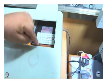
This is where the lamps are in this particular spectrophotometer if you can read the handwriting there are 2 lamps, W means tungsten lamp and the deuterium lamp. Tungsten provides visible wavelength and deuterium and provides ultraviolet wavelength. Now, you might be wondering what is the need of 2 lamps in the first place, we need 2 lamps because tungsten does not give ultraviolet and deuterium lamp is not good for visible source.
