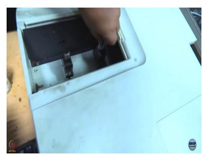
And now as you see, there are 2 places where you could keep your samples. This is called the sample compartment. This is called the reference compartment. And light comes out through these 2 holes and goes through these 2 and finally, there are 2 detectors there these 2 detectors record I0 and It respectively, and work out the absorbance. So, since we are using 2 detectors, it is important that we correct for their responses.
