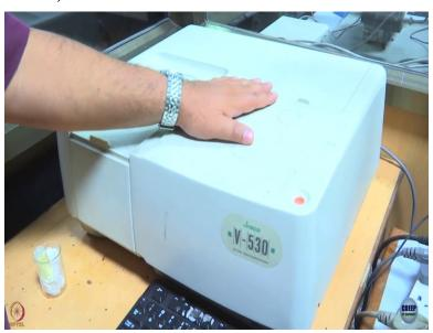
This is an absorption spectrophotometer. You might remember from the previous lecture, that it consists of a lamp, a source of light, a dispersing element and a slit, which combined is called the monochromator and then you have the sample and the detector.
