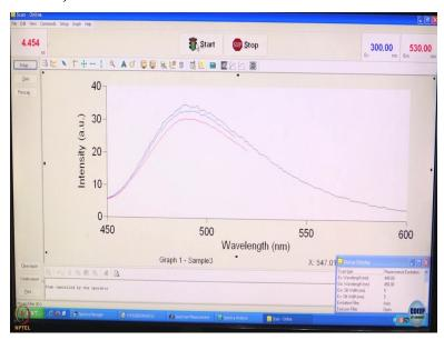
So this is our setup, I am now going to record an emission spectrum. So you can see the spectrum building right here, initially the intensity is very less. So zoom in a little bit now you can see the spectrum forming. And once again, it is forming point by point. Each point corresponds to a particular position of the emission monochromator and as you might see, the quality of spectrum is not very good, because I am doing it very quickly.
