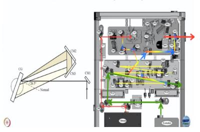
So PM1 first hit then it has gone to PM2 PM1 PM2 then from PM2 it goes through PL3 to PM3 from PM3 it goes straight through the Ti sapphire rod and while doing that it goes through one of these mirrors since it will covered I want you to read the name what is this? RM3 is a again dichroic mirror it allows green light to go through it going to reflect red light completely. So it goes straight okay then it is done so pumping of the regen is done.
