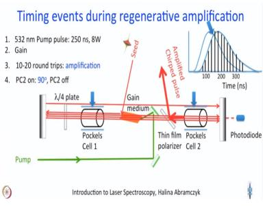
And in the last couple of modules we have discussed in as much detail as you could without getting into too much of instrumentation the timing events that are there during regenerative amplification. And this is the one design that we have talked about the design where the gain medium is in a cavity and then this seed is switched in to the cavity by using a lambda by 4 plate it is kept in the cavity via combination of the same lambda by 4 plate and a Pockels cell.
