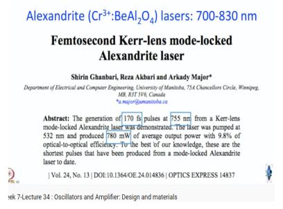
Another material that is used is called Alexandrite is chromium dope Bal2O4 the range of tunability the range of emission is 700 to 830 nanometer. In fact I think in 1979 or so the first tunable laser solid state was made using Alexandrite so it is been there in the market for long time
