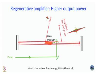
Now let is come to the design we have in our lab, it is called regenerative amplifier here you have higher output power. The difference between multi-pass amplifier and regenerative amplifier is that in a region the gain medium is actually inside a cavity. So, it is a laser by itself so, what you do is, these green mirrors are the pump mirrors. The black mirrors are the 2 mirrors of the laser. The point is both are high reflector mirrors there is no output coupler we have encountered this.
