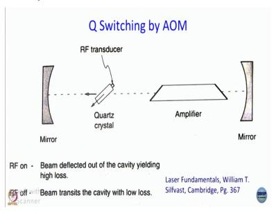
No, you can use our old friend acousto optic modulators as well. Not very difficult to understand use a Bragg cell any emission that comes will be sent off access by the Bragg cell most of the time. And then you can use a suitable frequency of sound, whenever it is favorable, the cavity will be switched on. So, you can do Q switching by AOM as well. EOM are more popular actually.
