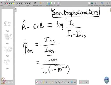
Epsilon CL and absorbance actually defined as log off  $I_0$  by  $I_t$  where I 0 is the intensity of the incident light I t is the intensity of the transmitted light and we also learned that for a non-reflecting, absorbing sample I t is simply I 0 - I abs I used the I abs is important quantity for us. Let me write it like that. They are also studied that for emission spectroscopy define something called phi em emission quantum yield, which is given by I em divided by I abs.
