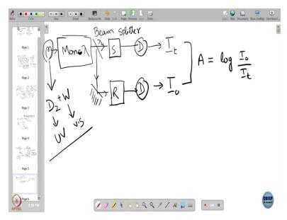
So what did we say we have light, we have sample and we will put the monochromator here, I want monochromatic, I want light of particular we are going to go through some lambda 1. So here and put in a monochromator. Since I am making a mess of it, I just write one more lambda n and of course, the lamp is somewhere here the lamp is the source of light. And remember, we are talking about absorption spectrophotometer here.
