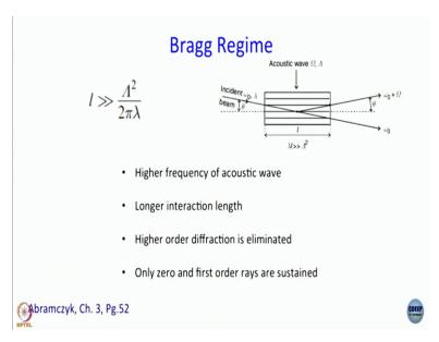
We have talked about mode locking, how you do mode locking using acousto optic modulator, that time we said that we have to use it, use it AOM in Raman Nath regime, where L was much less than lambda square by 2 pi small lambda capital lambda is the wavelength of sound wave, small lambda is the wavelength of light. In case of cavity dumping I think we have discussed it in the previous module as well.
