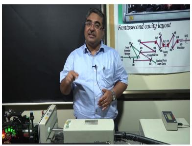
This is the pump mirror, as you said it is a diode pump solid state laser. The way it works is that under the table we have this diode banks, which have pigtail. Pigtail means there is an optical fiber that comes out from the end of the diodes themselves and that is what takes the light on to the active medium of the laser that is kept here. It is NDLF in our case, NDLF, like Nd YAG uses about 1064 nanometer which is IR light and this is the cavity of the laser.
