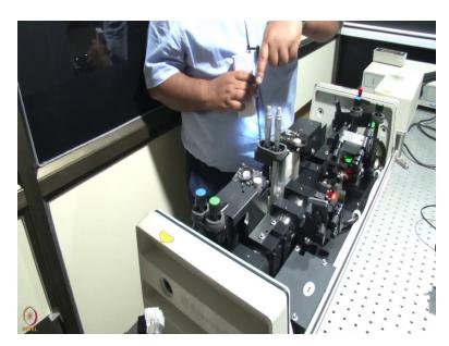
So, this is what the action is. This is the titanium Sapphire laser that gives us 100 femtosecond pulses tunable in principle from 700 nanometer to 950 or 1000 nanometers in practice, in this laser we have never gone beyond say 875 nanometer because once you go beyond 900 nanometer, then the moisture in the air starts creating a problem. And so you need to keep this entire laser cavity parsed in nitrogen and that nitrogen would better we dry nitrogen that is too much of a trouble.
